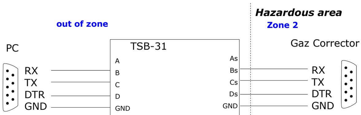
Note that RS-232 norm specifies that RS-232 voltage can be up to  $\pm 15\text{V}$ . With such voltage, the protection diodes will clamp the voltage and drain a high current and possibly blowing the fuse.
