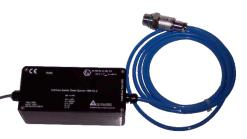
TPL-211 has two pressure sensors inputs.
